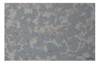
Fine particle of Titanium-based carbonitride is dispersed in bonded phase.
