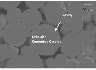
Granular cemented Carbide is formed, and about 100∼250µm of cavity exists between particles.
